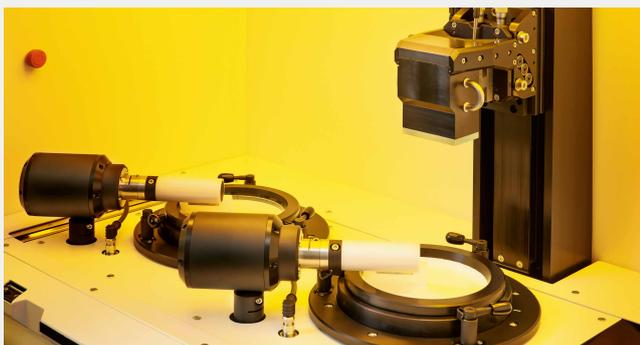
Additionally, two individually user-controlled platforms are included in the **ready to develop module**. The platforms can be customized, giving you for the first time the freedom to integrate own processes and technologies (e.g. ink jetting, coating, monitoring devices etc.) within a 3D printing job to drive innovation further than ever before.
